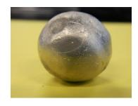
Encapsulated Phase change material for thermal Energy Storage System in Concentrated Solar Power Plant (CSP)
